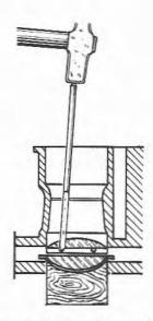
Fig. 7.20 Peening the throttle valve retaining screws (Sec 7)
