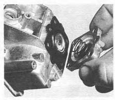
$6.12B\ ...$  and lift off the needle diaphragm cap and spring ...
