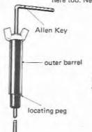
Fig. CDSE9 The special tool for adjustable needles
