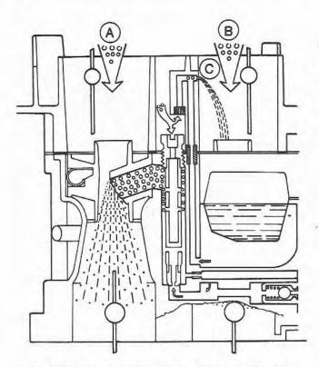
Fig. 10.3 Carburettor full power overfeed phase (Sec 3)
