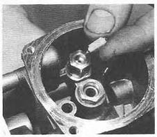
9.16A Removing the float needle
