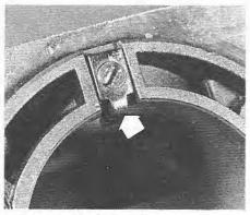
9.9 Piston guide (arrowed)
