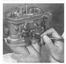
5.22 Tighten the carburetor-to-intake manifold bolts
