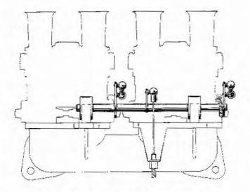
Fig. 2.6 Typical cable and rod throttle control
