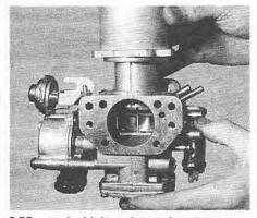
9.58 ... and withdraw the suction chamber and piston assembly
