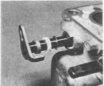
5.55 Showing the correct location of the secondary throttle shaft spacer, seal and washer
