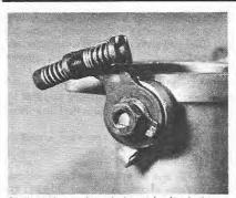
8.12 Fitting a throttle lever (twin choke type)
