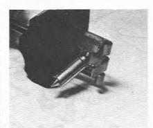
5.8 Position of the needle valve on the float assembly
