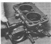
5.51 Removing the primary throttle shaft (DFAV type)
