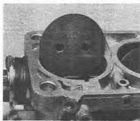
5.36 Removing a throttle valve
