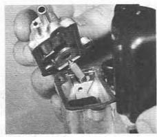
6.8B ... and withdraw the float chamber cover
