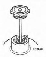
Fig. 8.11 Piston damper guide clip position (Sec 9)
