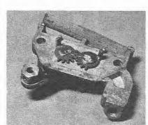
5.23 Removing the starter device air filter gauge, also showing sector alignment marks
