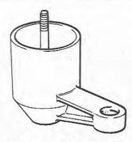
Fig. 4.20 SU type H float chamber
