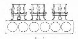
Fig. 11.4 Three carburettors fitted to a six-cylinder in-line engine (Sec 1)
