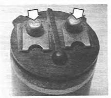
5.10B Solenoid terminals (arrowed)
