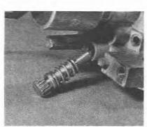
5.30 Idle mixture adjusting screw
