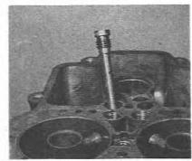
5.23a Removing the starting jet assembly
