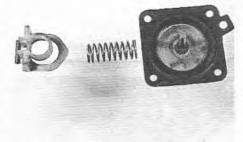
13.11 Accelerator pump diaphragm components
