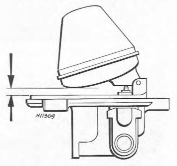
Fig. 7.8 Float level setting - all-plastic type (Sec 8)
