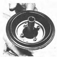
10.12b Tighten the four screws progressively
