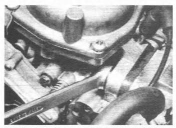
Fig. 3.5 Check the carburetor mounting bolts for the correct torque
