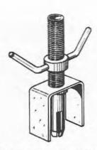
Fig. 6.9 Auxiliary venturi removing tool (Sec 5)
