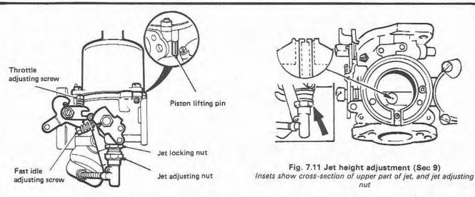
Fig. 7.10 HS carburettor adjustment points (Sec 9)
