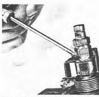
8.14 Bend back the locking lip carefully to enable its re-use
