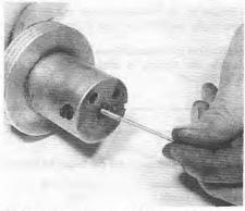
7.5 Removing the needle from the piston
