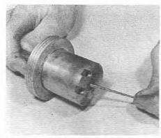
7.6B ... and withdraw the needle
