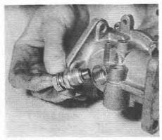
7.13 Removing the jet locking and adjusting nuts
