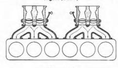
Fig. 11.5 Two carburettors fitted to a six-cylinder in-line engine (Sec 1)
