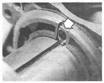
8.8 Piston key (arrowed)
