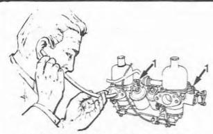
Fig. 5.11 Balancing twin carburettors (Sec 9)
