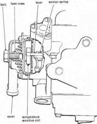
Fig. CDST4 Another cross-sectional view of the automatic starter
