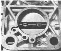
5.42 Primary throttle valve and retaining screws
