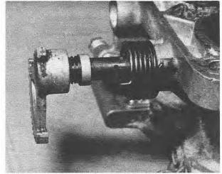
6.50 Removing the secondary throttle shaft (DGAS type)
