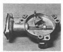
9.23 Fitting the automatic choke shaft (DGAS type)
