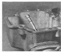
5.13 The accelerator pump discharge blanking needle
