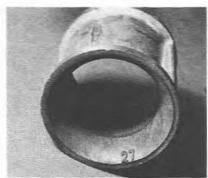
5.33 Typical choke, showing diameter identification mark
