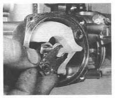
9.13B ... and withdraw the jet and adjusting lever assembly
