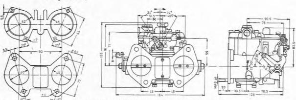
Fig. 11.6 Overall dimensions of the DCOE carburettor (Sec 2)
