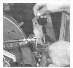
5.28 . . . finally install the right side air horn assembly gasket
