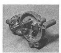
5.33 Removing the automatic choke shaft (DFAV type)
