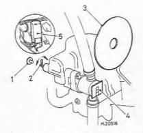
Fig. 8.14 Adjusting the FASD (Sec 12)
