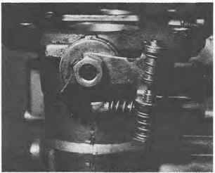
7.9 Throttle lever fitted to the spindle
