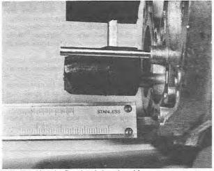
7.41 Checking the float level closed position
