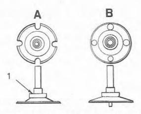
Fig. 6.2 Standard (A) and Rolls Royce (B) jets for the HD carburettor (Sec 3)
