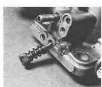
5.19 Removing the idling mixture adjusting screw
