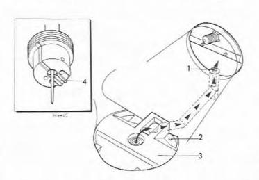
Fig. 8.8 Bypass idle system (Sec 7)
