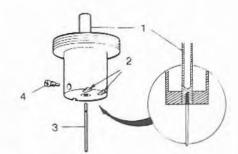
Fig. 6.4 Piston and needle components (Sec 6)
