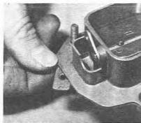
5.20 Removing the cover dust seal (DFAV type)
