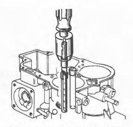
Fig. 7.14 Reaming the emulsion tube bores (Sec 6)
