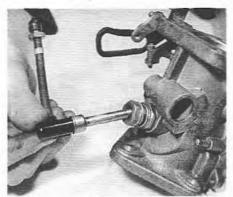
7.12 Removing the jet assembly
