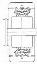
Fig. 8.1 Two carburettors fitted to a 4-cylinder opposed engine (Sec 1)
