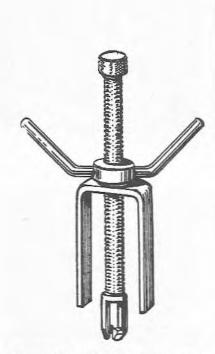
Fig. 11.13 Auxiliary venturi extracting tool (Sec 5)
