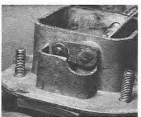
9.52 Fitting the choke operating lever (DGAS type)
