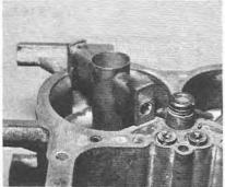
6.38 Removing the auxiliary venturi (DGAS type)
