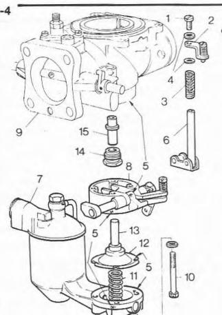
Fig. 6.3 Type HD jet housing components (Sec 6)
