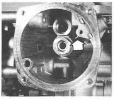
9.17A Jet bearing and locking nut location.
