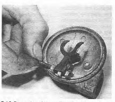
7.12 Removing the needle valve hinge pin and lever
