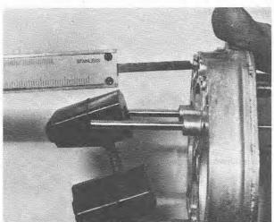
7.42 Checking the float level open position
