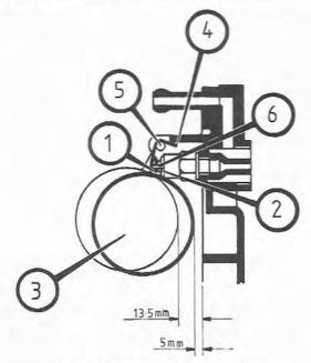
Fig. 6.16 Float level adjustment (Sec 7)
