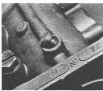
5.31 Progression hole inspection screw plug location
