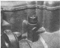
5.19a A pump jet retaining screw
