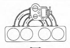
Fig. 6.1 Single carburettor fitted to a four-cylinder in-line engine (Sec 1)
