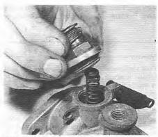
7.9A Removing the jet locking nut ...
