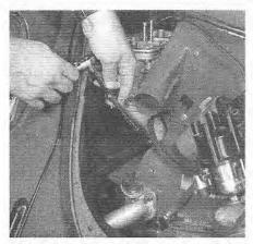
5.24 Tighten the manifolds onto the cylinder heads using a speed wrench and extensions
