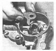
4.5 Dismantling: Note the catch hole for the spring end
