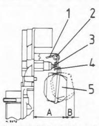
Fig. 7.21 Checking the float level adjustment (DFV, DFAV, DGV, DGAV types) (Sec 7)
