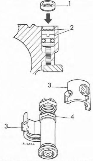
Fig. 7.4 Tamperproof cap and clamp fitted to later models (Sec 2)
