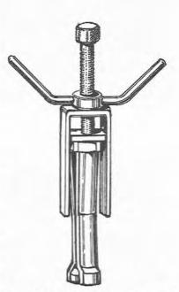
Fig. 11.14 Choke extracting tool (Sec 5)
