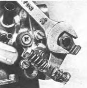
9.6 Main assembly: Note the positions of the springs
