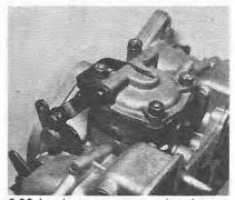
6.20 Accelerator pump cover location (triple choke type)
