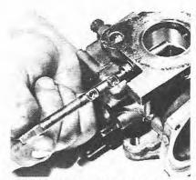
8.9b Withdraw the spindle at right angles
