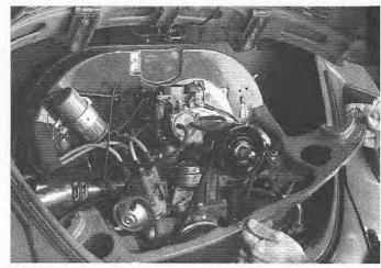
5.5 Remove the cooling tin breast plate
