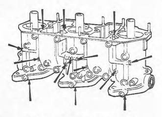
Fig. 8.15 Lead plug location points (Sec 7)
