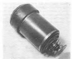
5.6B Solenoid and spring-tensioned disc
