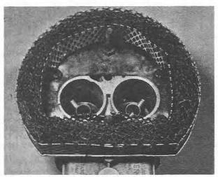
2.0 Typical air cleaner with the cover removed
