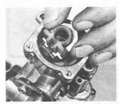
13.10A Removing the plastic guide/valve
