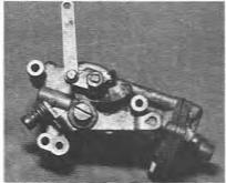
9.26 Fitting the fast idle lever (DGAS type)
