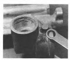
5.6C Removing the clip from the pivot
