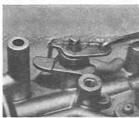
5.34a Removing the automatic choke
