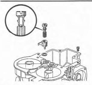
Fig. 9.17 Location of the acclerator pump ball valve (Sec 7)
