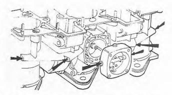
Fig. 8.16 Accelerator pump channel lead plug location points (Sec 7)
