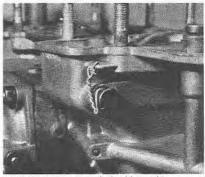
9.32 Float fulcrum pin locking wire location (triple choke type)
