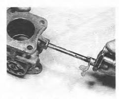
6.18 Throttle spindle removal
