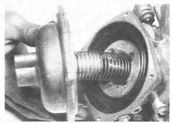
Fig. 4.24 Suction chamber cover on a Stromberg carburetor
