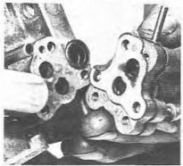
6.11 Note the positioning and the gasket
