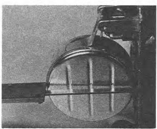
7.43 Checking the float open position with vernier calipers
