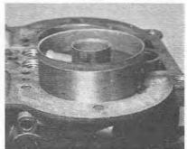
7.21c Fitting an auxiliary venturi
