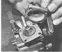
5.10a Withdrawing the accelerator pump cover  $\dots$
