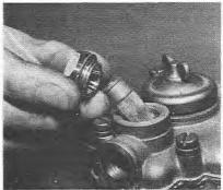
5.2 Removing the fuel filter
