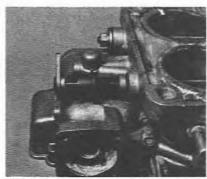
6.44 Withdrawing the primary throttle shaft (DGAS type)
