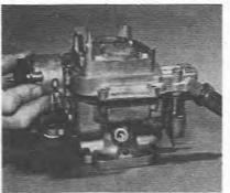
5.3 Lifting the carburettor cover
