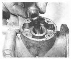
6.10 Jet locking nut and bearing removal
