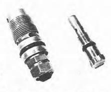
8.10a The two parts split once out of the body; note the O rings
