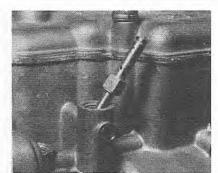
5.19b Removing a pump jet
