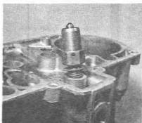
5.7 Removing the needle valve (twin choke type)
