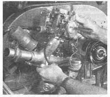
5.13 ... lift the carburetor/intake manifold assembly from the engine
