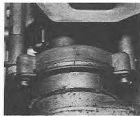
8.66 Automatic choke alignment marks (DFAV type)
