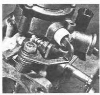
4.2 Removal: Keep out the fast idle lever from the Autostarter
