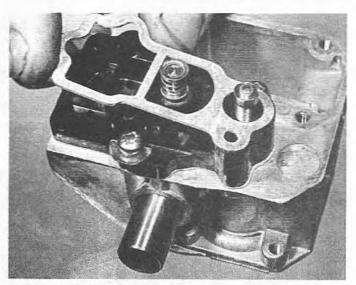
6.16 Removing the top cover gasket
