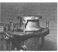
6.27a Removing a choke (triple choke type)
