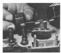
5.4b Removing the float and needle
