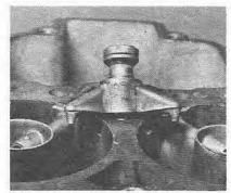
5.11 Removing the accelerator pump delivery valve and jet
