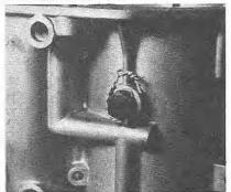
9.19 Locking wire attached to the choke retaining screw (triple choke type)
