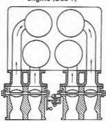
Fig. 11.3 Two carburettors fitted to a four-cylinder V-engine (Sec 1)
