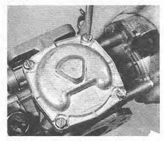
9.12A Removing the float chamber cover screws
