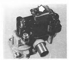
11.21 Bi-metal unit (arrowed)
