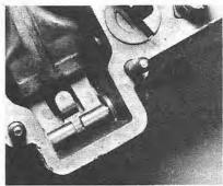
8.26 Fitting the float (twin choke type)
