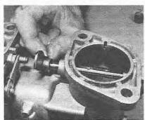
8.4 Fitting the throttle shaft (twin choke type)
