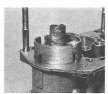
5.22 Removing an auxiliary venturi
