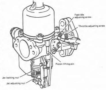
Fig. 5.7 Type H carburettor tuning points (Sec 9)
