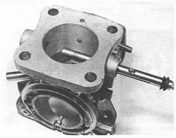
9.21A Removing the throttle spindle
