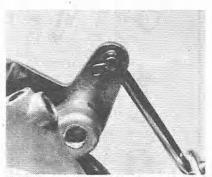
5.12 Starter device operating rod split pin location
