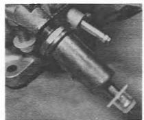
5.2 Removing the fuel filter
