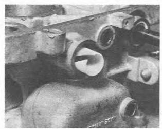
5.56 Removing a Tefion bush from the secondary throttle shaft bore
