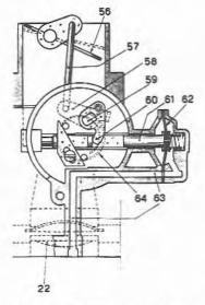
Fig. 7.3 Automatic choke operation (Sec 3)
