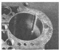
7.21a The choke and auxiliary venturi locating groove
