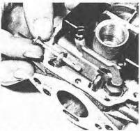
8.13 No force should be necessary to withdraw the float hinge pin
