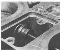
7.13 Fitting the accelerator pump lever fixing pin
