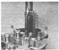
Fig. 8.19 Fitting the accelerator pump (twin choke type)
