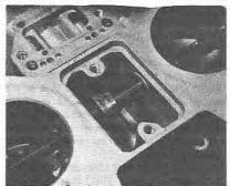
7.4b Fitting the throttle spindle
