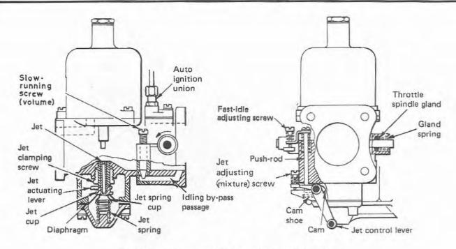
Fig. 6.1 Cutaway view of the Type HD carburettor (Sec 2)
