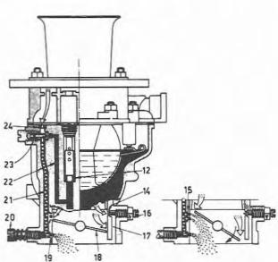
Fig. 8.4 Idling and progression phase (triple choke types) (Sec 3)
