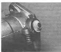
7.6 Fitting a throttle spindle dust cover
