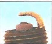
Symptoms: Rounded electrodes with a small amount of deposits on the firing end. Normal color. Causes hard starting in damp or cold
