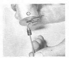
7.6C Removing the spring-loaded type needle
