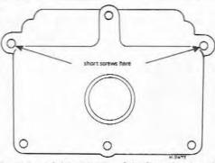
Fig. CD6 View of the underside of the float chamber, showing the order of tightening of the fixing screws
