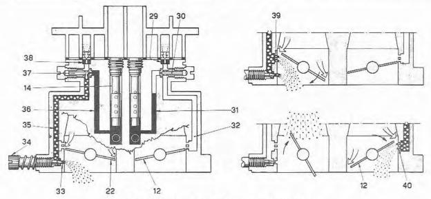
Fig. 7.4 Carburettor idling and progression phase (Sec 3)
