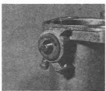
5.30 Removing the spring retainers (twin choke type)
