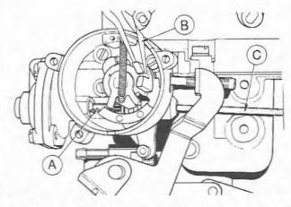
Fig. 10.8 Checking the vacuum pull down adjustment (Sec 8)
