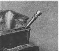
6.18 Removing the discharge blanking needle (DGAS type)
