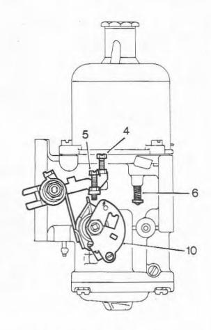
Fig. 8.15 Manual choke HIF carburettor tuning points (Sec 14)
