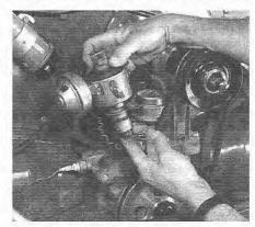
5.14 Remove the stock distributor from the engine
