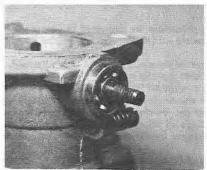
7.5 Fitting a spindle bearing
