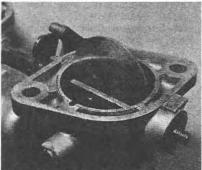
5.27 Removing a throttle valve (twin choke type)
