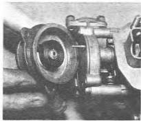
5.25 Withdrawing the thermostat housing (DFAV type)
