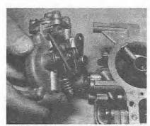
8.30a Fitting the automatic choke body (DFAV type)
