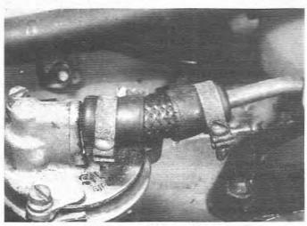
Fig. 3.1 Checking the fuel supply hose on a SU carburetor
