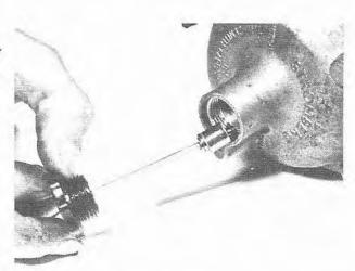
8.1 This is how the damper is removed
