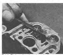
7.14 Fitting the throttle spindle return spring anchoring plate
