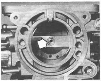
14.8B Upper view of the jet (arrowed)
