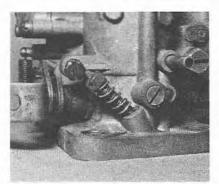
5.18 Removing the idling mixture adjusting screw
