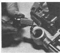
5.5 Removing the fuel filter and plug
