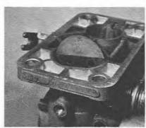
5.36 Removing the secondary throttle valve
