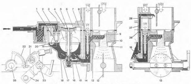
Fig. 9.6 Carburettor normal phase (DGAS types) (Sec 3)
