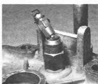
5.7 Removing the needle from the needle
