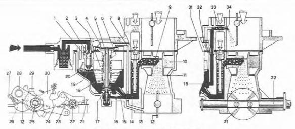
Fig. 7.6 Carburettor normal phase (Sec 3)
