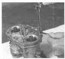
5.17 Double nut the studs for removal
