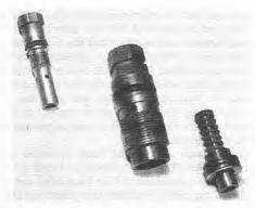
Fig. 4.12 Complete jet assemblies on a typical Stromberg carburetor
