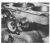
5.51 Removing the secondary throttle shaft nut
