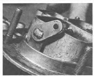
7.43 Choke lever position with the valves shut
