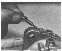
5.28 Removing an air bypass screw
