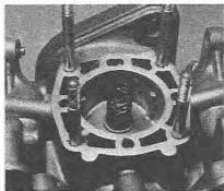
9.21 Correct location of the accelerator pump reaction spring (triple choke type)
