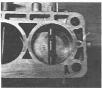
5.48 Throttle valve retaining screw location (DFAV type)
