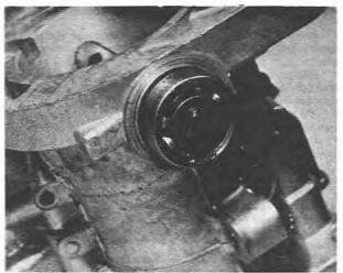
7.9 Fitting the throttle spindle bearing
