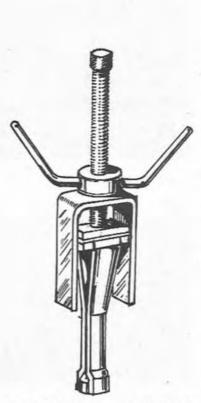
Fig. 8.11 Choke removal tool (Sec 5)
