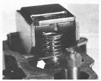
6.15 The bi-metal unit (arrowed) is located beneath the spring
