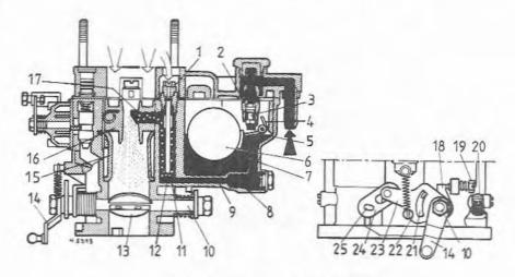
Fig. 6.5 Carburettor normal phase (Sec 3)
