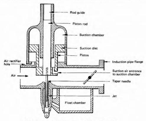
Fig. 1.12 The basic SU carburetor in simplified cross-section
