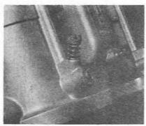
5.21 Idling mixture screw location (twin choke type)
