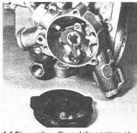
4.4 Dismantling: Record the position of the components
