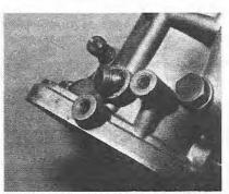
6.42 Removing the progression hole inspection plugs (triple choke type)
