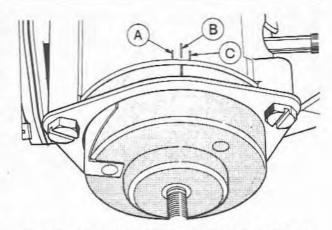
Fig. 10.7 The automatic choke alignment marks (Sec 7)
