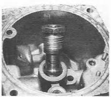
9.17B Removing the jet bearing and locking nut
