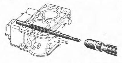
Fig. 7.16 Reaming the throttle shaft bore (Sec 6)
