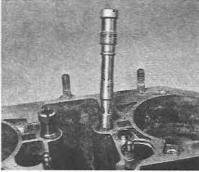
5.12 Removing an emulsion tube (twin choke type)
