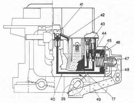
Fig. 7.7 Carburettor acceleration phase (Sec 3)
