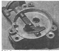
5.34 Removing the stop plate (DFAV type)
