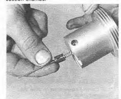
9.88 ... and withdraw the needle, guide and spring
