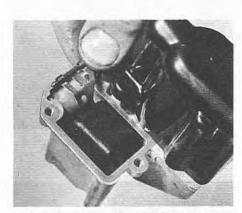
6.10 Lifting the float from the float chamber
