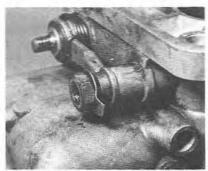
5.38 Removing a primary shaft retaining nut
