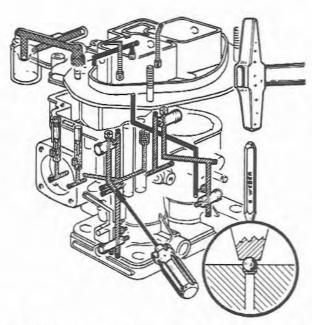
Fig. 7.17 Location of the carburettor internal channels and method of fitting the lead plugs (Sec 6)
