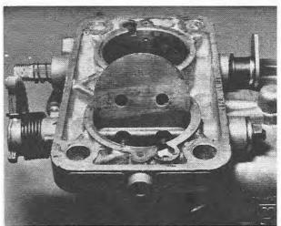
6.47 Removing a throttle valve (DGAS type)
