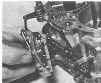
5.13 Removing the starter device
