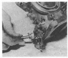
7.21 Spindle nut removal
