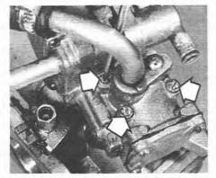
13.5A Remove the through-bolts (arrowed)
