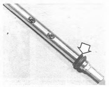
9.21B Throttle spindle and seal (arrowed)
