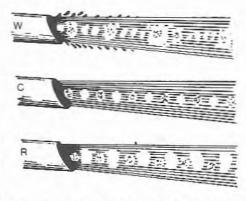
Fig. 5.9 Diagram of effect on exhaust of mixture strengths at idle speed (Sec 9)
