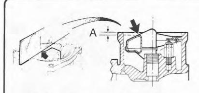
Fig. 8.12 Checking the float level dimension (Sec 10)
