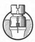
Fig. 7.12 Using the special tool to hold the throttle shaft stationary (Sec 5)
