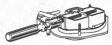
Fig. 7.15 Reaming the choke shaft bore (Sec 6)
