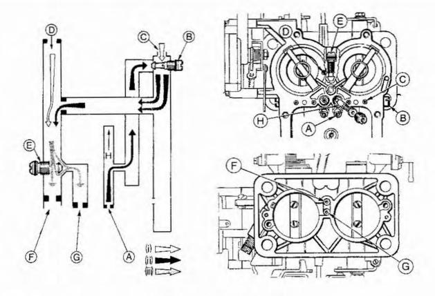
Fig. 1.14 The Weber bypass idle system
