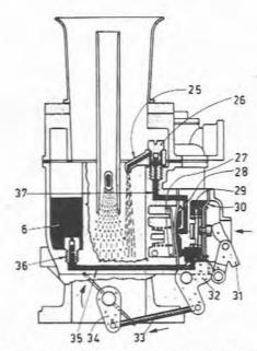
Fig. 8.8 Acceleration (triple choke types) (Sec 3)
