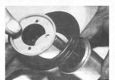
Fig. 4.26 Removing the diaphragm on a Stromberg
