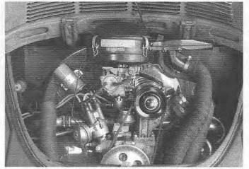
5.4 The project engine is a mostly stock VW 1600 engine with dual port heads
