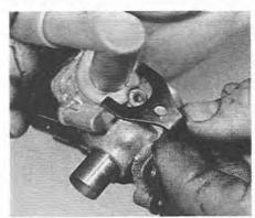
11.19A Air inlet stub and clamp removal
