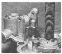
5.9 Removing the needle valve seating
