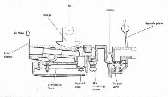
Fig. CDSE3 Horizontal cross-section through the choke bore, showing the arrangement of the temperature compensator, idle trimming screw and by-pass valve
