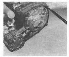
11.13 Removing the ASU-to-carburettor adaptor plate screws
