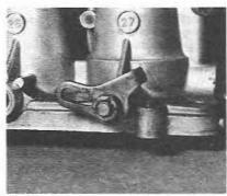
5.49 Secondary throttle lever components
