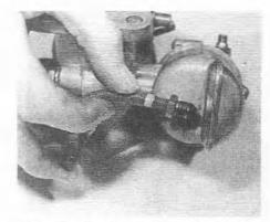
7.10 Jet feed pipe removal from the float chamber
