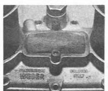
5.2 Removing the filter gauze (twin choke type)
