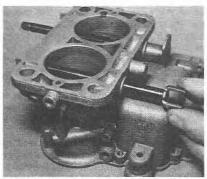
5.50a Removing a throttle shaft (DFAV type)
