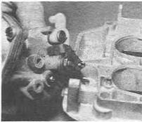
5.11 Disengaging the electric choke lever
