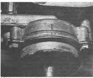
9.64 Automatic choke alignment marks (DGAS type)
