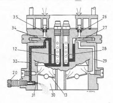
Fig. 6.4 Carburettor idling and progression phase (Sec 3)
