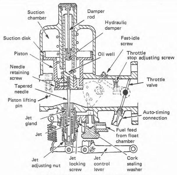
Fig. 5.1 Cross-section through the type H carburettor (Sec 2)
