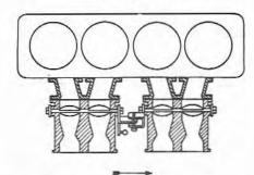
Fig. 11.2 Two carburettors fitted to a four-cylinder in-line engine (Sec 1)
