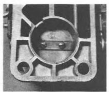
5.35 Location of the secondary throttle valve retaining screws
