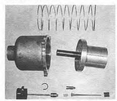
9.8C Piston and suction chamber components
