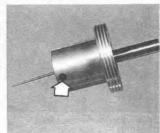
9.8A Unscrew the needle guide locking screw (arrowed) ...
