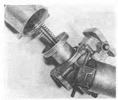
6.3 Removing the suction chamber
