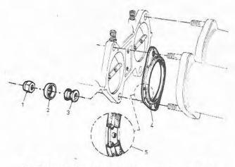
Fig. 11.11 Anti-vibration mounting components (Sec 4)
