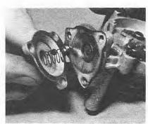
5.38 Removing the automatic choke diaphragm cover and spring (DFAV type shown)
