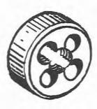
Fig. 4.4 Typical thread die
