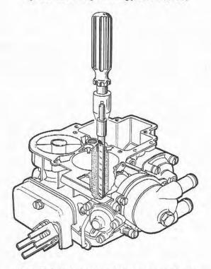
Fig. 9.13 Reaming the emulsion tube bores (Sec 7)
