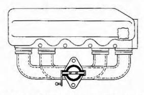
Fig. 2.2 Correct location of a single carburetor feeding four cylinders, showing the position of the throttle spindle
