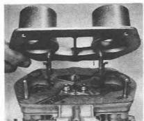
5.2 Removing the air horns
