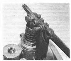
7.6B Removing the lever clevis pin
