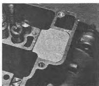
5.6 Location of the carburettor bowl baffle plate
