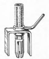
Fig. 9.11 Tool for removing the auxiliary venturis (Sec 6)
