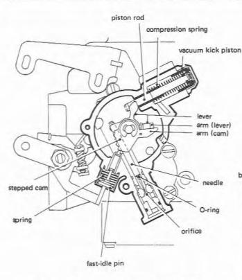
Fig. CDST3 Side cross-section of the thermostatically controlled automatic starter
