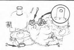
Fig. 5.12 Control couplings on multiple carburettor installations (Sec 9)
