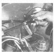
5.35 Tighten the union piece to allow maximum linkage travel
