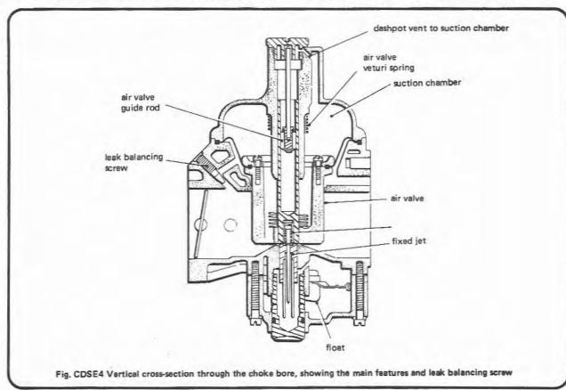
spurious leak. Once the screw is set, on initial build, it must not be altered and to prevent tampering, the bore into which it fits is sealed with a plug. The body, air valve and cover become a matched set and neither part may be replaced independently of the other. The suction chamber cover is wired to the body, and may only be removed after a seal has been broken, thus revealing that the unit has been tampered with.
