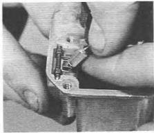
6.9 Releasing the float needle from the float
