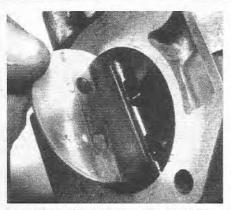
Fig. 4.10 Throttle plate on a SU carburetor
