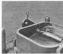
5.3 Disconnecting the choke operating rod
