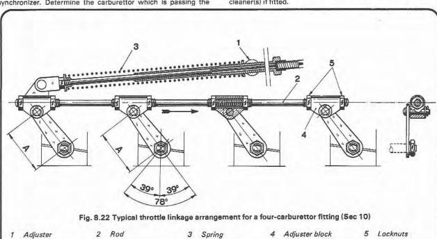
Note: Dimensions A and lever angles must all be identical
