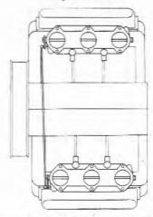
Fig. 8.2 Two carburettors fitted to a 6-cylinder opposed engine (Sec 1)
