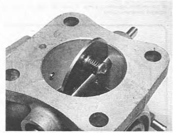
10.6 Inserting the throttle disc
