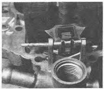
5.5a Withdrawing the float fulcrum pin ...
