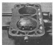
5.49a Removing a throttle valve (DFAV type)
