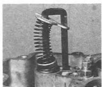
5.20 Removing the accelerator pump assembly
