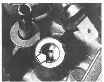
14.8A Mixture adjusting screw location (arrowed)
