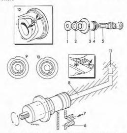
Fig. 8.3 Cold start enrichment device (Sec 5)
