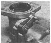
5.28 Accelerator pump lever location (twin choke type)
