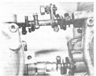
Fig. CD10 Twin carburettor multiple connections
