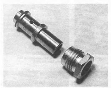
9.17C Locking nut separated from jet bearing
