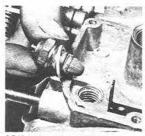
6.9 Make sure the gauze filter on the needle valve is clear
