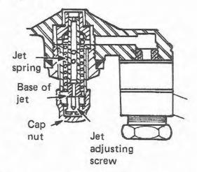
Fig. 5.4 Cross-section of the thermostatic carburettor jet (Sec 3)
