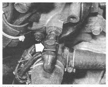
14.14 Coolant thermistor wiring plug (arrowed)
