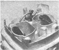
5.19 Choke link locations on the carburettor cover
