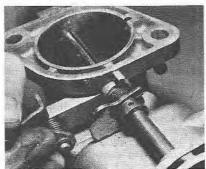
8.7 Correct location of the accelerator pump cam (twin choke type)
