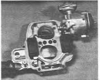
7.67 Float assembly location on the carburettor cover
