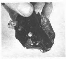
13.6D Removing the gasket from the delay valve
