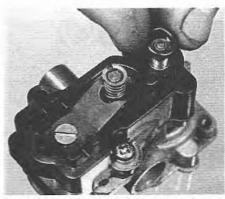
11.22 Fuel metering needle O-ring removal
