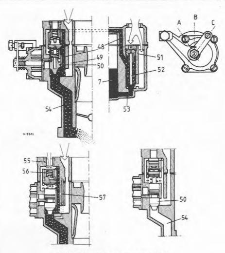
Fig. 6.3 Cold starting device operation (Sec 3)
