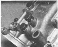
6.13 Removing the drain plugs (triple choke type)
