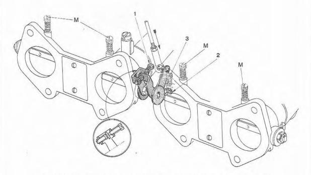
Fig. 11.24 Linked throttle accelerator rod arrangement on a dual carburettor fitting (Sec 8)
