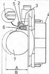
Fig. 13.6 Float level adjustment dimensions (Sec 7)
