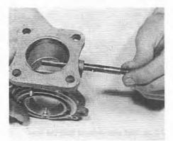
7.22 Removing the throttle spindle
