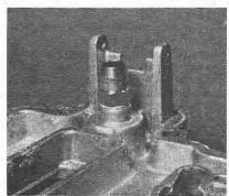
7.38 Needle valve seating location in the carburettor cover
