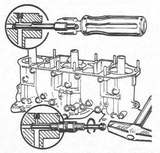
Fig. 8.14 Overhauling the idling jet seats (triple choke types)
