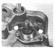
9.26A Remove the screws (arrowed) ...
