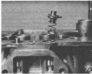
7.31 Fitting a starter valve spring, retainer and spring washer
