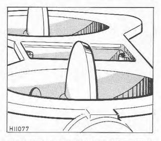
Fig. 11.19 Angled perimeter of the throttle valves (Sec 7)
