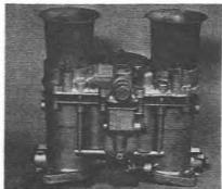
5.5 Removing the carburettor cover (twin choke type)
