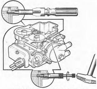
Fig. 9.12 Reforming the idling jet seats (Sec 7)
