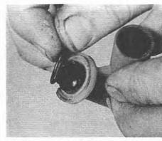
11.19B Air inlet stub O-ring removal
