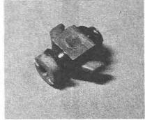
5.19b The accelerator pump valve and let
