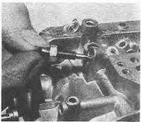
5.28 Removing an air bypass adjusting screw
