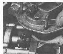
5.4 Removing the carburettor cover (DFAV type shown)
