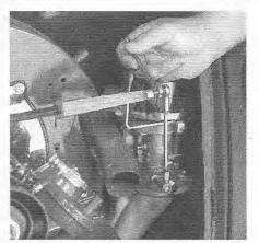
5.31 Tightening the upper linkage arm adjustment nut
