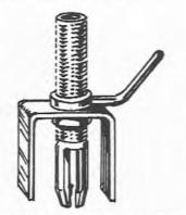
Fig. 8.10 Auxiliary venturi removal tool (Sec 5)
