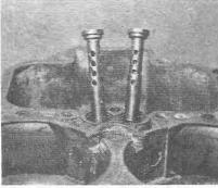
6.13a Removing the emulsion tubes (DGAS type)
