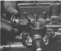
5.2 Removing the fuel filter (DFAV type)
