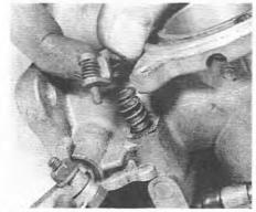
6.8 Removing the fast idle adjustment screw plate
