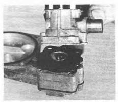
11.16 Removing the ASU from the adpator plate
