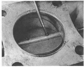
8.2 Spreading the throttle disc screw split ends
