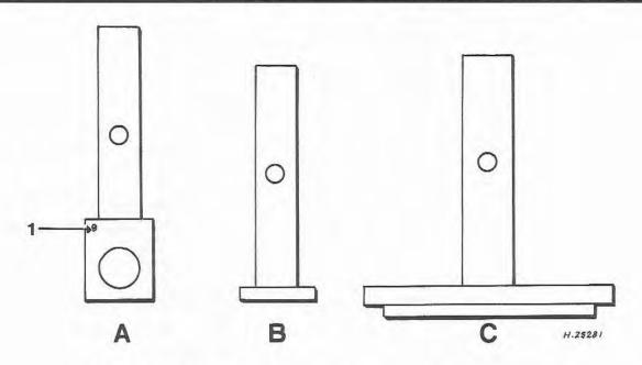
Fig. 5.2 The three types of jet - Standard (A), Thermostatic (B), and Invicta (C) (Sec 3)
