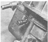
6.11a Removing an idling jet (DGAS type)
