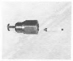
9.16C Needle valve seat and float needle
