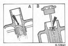
Fig. 8.13 Piston damper oil level (Sec 10)
