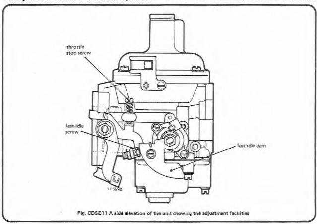
assembly and consequent damage to the diaphragm, the Allen key may be turned a maximum of one turn in either direction to set optimum idle quality (smooth, even running with colourless exhaust and no 'hunting').
