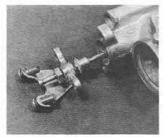
5.8A Removing the needle valve assembly
