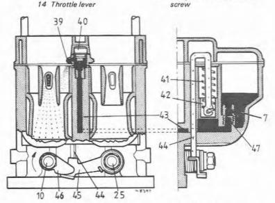
Fig. 6.6 Carburettor acceleration phase (Sec 3)
