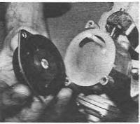
5.9a Removing the electric choke housing
