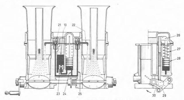
Fig. 8.7 Acceleration phase (46 IDA and 48 IDA) (Sec 3)
