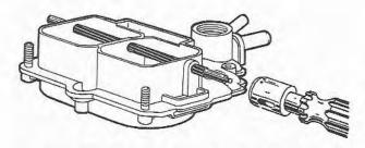
Fig. 9.14 Reaming the choke shaft bore (Sec 7)
