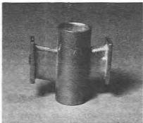
5.32b An auxiliary venturi showing size identification
