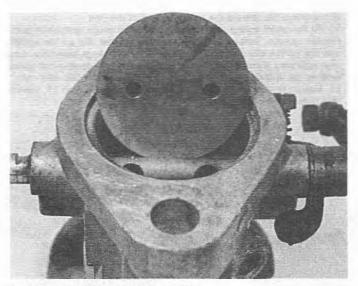
7.15B ... and withdraw the throttle disc ...
