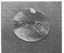
5.49b Throttle valve showing the idle bleed hole (DFAV type) (arrowed)
