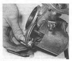
7.11A Removing the float chamber lid ...
