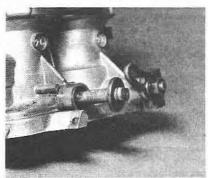
5.45 Removing the primary throttle shaft spacer
