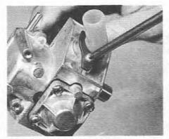
6.6 Removing the hot air inlet stub
