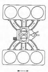
Fig. 9.2 Single carburettor fitted to a six-cylinder V-engine (Sec 1)
