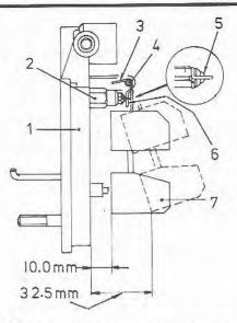
Fig. 12.7 Float level adjustment dimensions (Sec 7)
