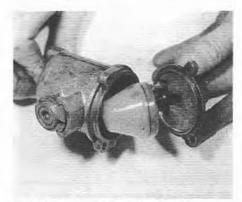
7.16 Removing the float chamber lid
