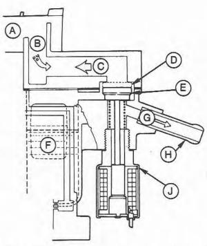
Fig. 10.4 Float chamber vent valve operation (Sec 3)
