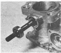
5.39 Removing the throttle spindle
