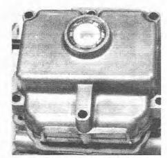
Fig. 4.17 Float chamber on a typical Stromberg carburetor
