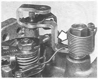
9.19A Throttle return spring (arrowed)
