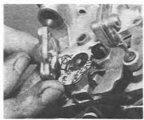
5.28a Lifting off the power valve cover, spring ...
