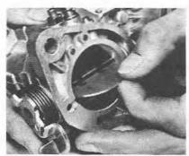
5.33 Removing a throttle valve
