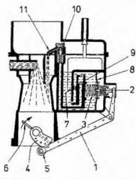
Fig. 1.8 The Weber diaphragm type accelerator pump
