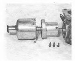
7.4 Removing the suction chamber
