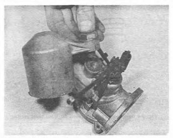
7.14 Removing the float chamber
