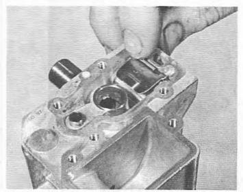
6.20 Checking air valve movement
