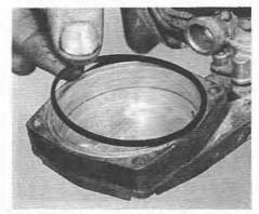
11.14A Removing the upper O-ring ... -
