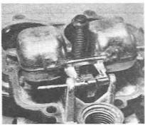
6.5 Withdrawing the float fulcrum pin (DGAS type)
