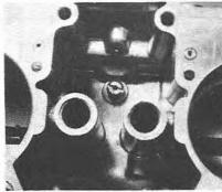
5.13 Accelerator pump inlet and discharge valve location
