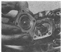
5.21 Withdrawing the accelerator pump cover
