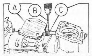
Fig. 8.20 Drilling the throttle spindle (triple choke types) (Sec 9) B Drill C Arm
