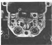
7.32 Fitted position of the accelerator pump
