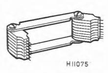
Fig. 4.2 Set of micron plug jet gauges
