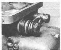
5.41 Removing the secondary shaft retaining nut
