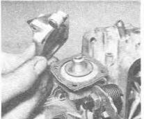
5.24a Removing the accelerator pump cover ...
