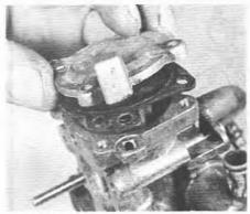
13.8 Accelerator pump diaphragm cover removal
