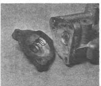
5.35 Removing the diaphragm cover (DFAV type)
