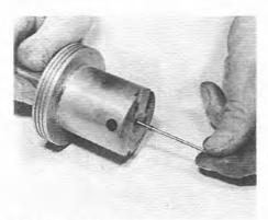
6.5B ... and withdraw the needle
