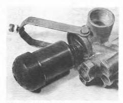
5.6A Removing the solenoid
