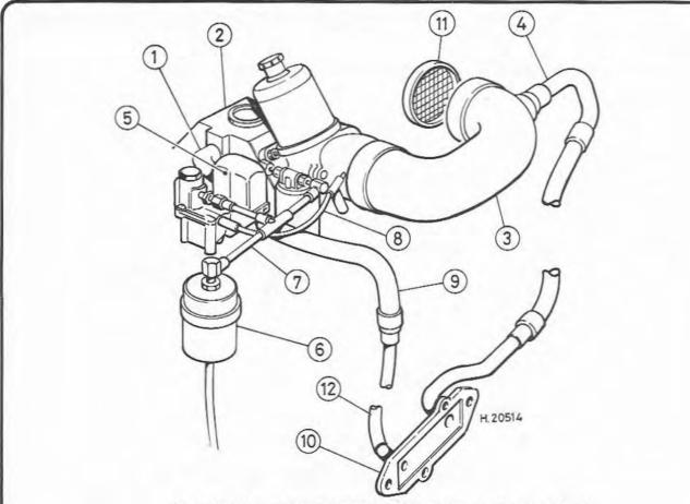
Fig. 9.7 Typical automatic enrichment device (AED) installation (Sec 6)
