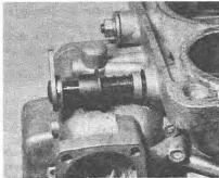
9.8 Inserting the primary throttle shaft (DGAS type)
