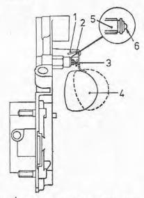
Fig. 9.21 Float level adjustment diagram (34 DGAS and DGAS types) (Sec 9)
