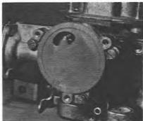
6.26 Insulation disc gasket location (DGAS type)
