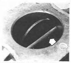
6.17A Showing the split ends of the throttle disc retaining screws (arrowed)
