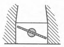
Fig. 7.23 Fast idle throttle opening checking location (Sec 8)
