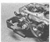
9.14 Fitting the sector adjustment screw (DGAS type)
