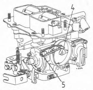
Fig. 7.24 Checking the automatic choke shaft setting on DGAV type carburettors (Sec 8)
