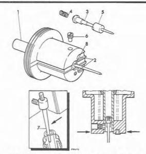
Fig. 8.4 Piston and needle components (Sec 6)
