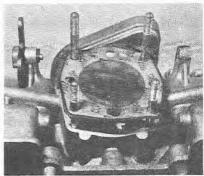
9.22a Fitting the accelerator pump release diaphragm ...
