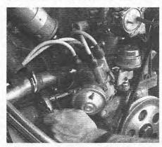
5.12 Remove the intake manifold center bolt and . . .
