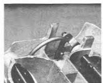
7.47 Correct fitted position of the choke
