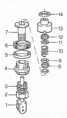
Fig. 5.3 Exploded view of the Standard jet components (Sec 3)
