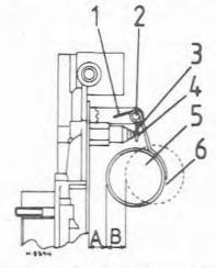
Fig. 7.22 Checking the float level adjustment (DFD, DFE, DFM, DIF, DAF types) (Sec 7)
