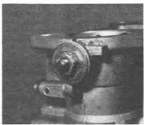
5.31 Throttle spindle outer retaining nut and locktab
