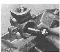
6.10 Removing the needle valves (triple choke type)
