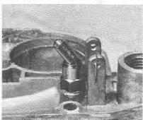
5.8 Removing the needle from the needle valve seating
