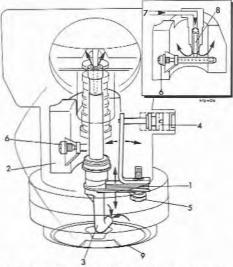
Fig. 8.1 HIF carburettor float chamber layout (Sec 2)
