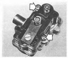
11.23 Valve body securing screws
