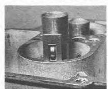
7.32 Inserting an auxiliary venturi
