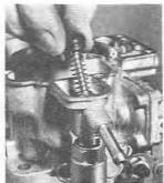
5.27b Removing the vent solenoid valve (USA types)
