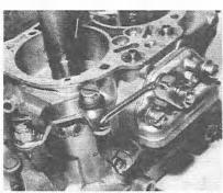
5.10 Starter device operating rod and lever location
