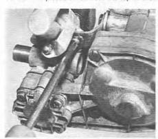
11.12 Removing ASU upper support bracket screw
