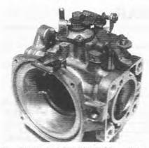
Fig. 4.5 Typical Stromberg CD carburetor body
