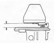
Fig. 7.7 Float level setting - steel arm type (Sec 8)
