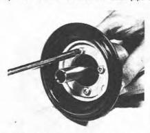
6.4 Note the Phillips head screws on the diaphragm
