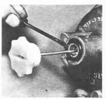
9.10a Main assembly: Finally the locating and fixing of the damper rod
