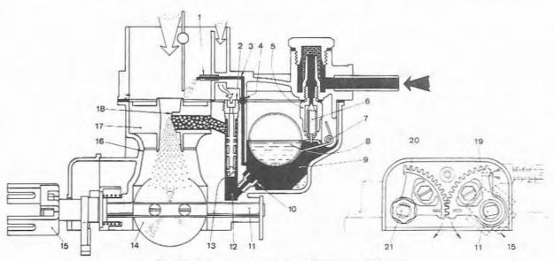
Fig. 9.5 Carburettor normal phase (DFAV types) (Sec 3)
