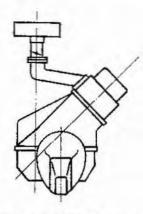
Fig. 2.3 The length of horizontal inlet manifold on this arrangement may cause carburetion problems when cornering
