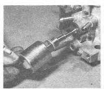
5.26 Removing the idle cut-off valve
