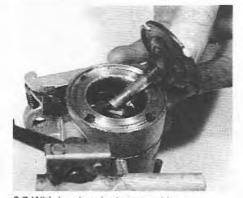
6.7 Withdrawing the jet assembly
