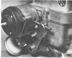
8.11 Showing the throttle lever and the fast idle adjusting screw
