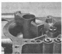
5.39a Removing the auxiliary venturi (DFAV type)
