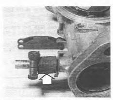
8.10 Throttle return spring (arrowed)
