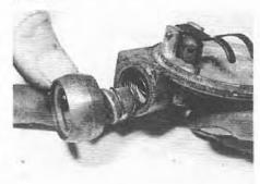
6.12 Removing the banjo inlet and filter from the float chamber lid
