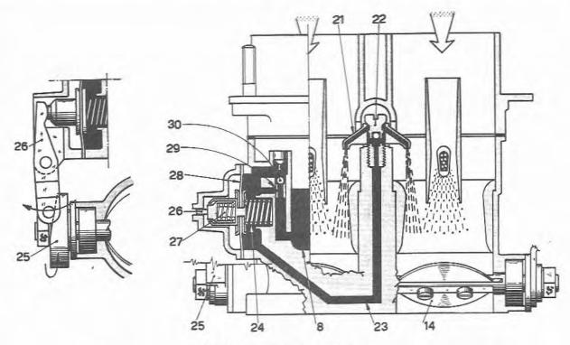
Fig. 13.4 Acceleration phase (Sec 3)
