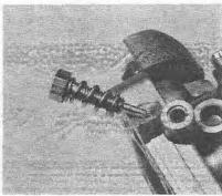
5.26 Removing an idling mixture adjusting screw
