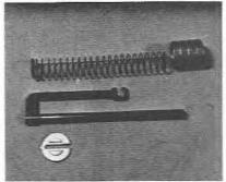
5.17 Accelerator pump components (twin choke type)
