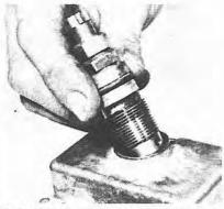
8.10 This shows the whole jet assembly being withdrawn
