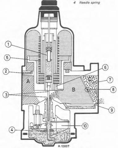
Fig. 8.5 Diagram of HIF carburettor operation (Sec 7)
