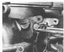
6.34 Accelerator pump cam location (triple choke type)
