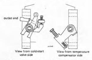
Fig. CDSE6 View of each end of the throttle spindle showing levers and springs
