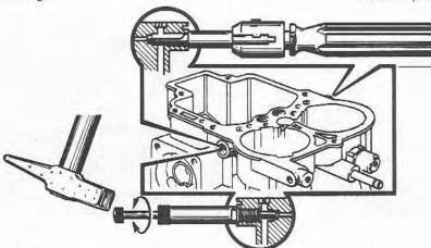
Fig. 7.13 Overhauling the idling jet seats (Sec 6)
