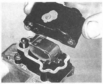
6.14B ... and separate the top cover from the valve body
