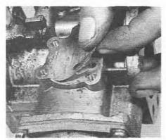
13.6B Peel the gasket from the carburettor
