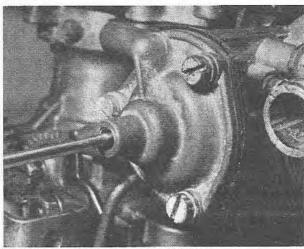
9.58 Adjusting the rod stop screw (DGAS type)
