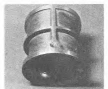
9.18 The choke and locating hole (triple choke type)
