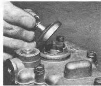
5.4 Removing the jet inspection cover
