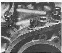
5.27 Removing a blanking screw
