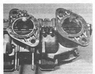
9.14 Fitting the intermediate linkage (triple choke type)
