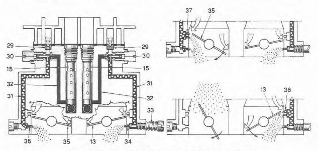
Fig. 7.5 Carburettor idling and progression phase (twin function) (Sec 3)
