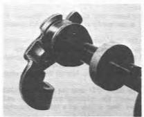
7.3a Crankcase emission rotary disc locating peg ...
