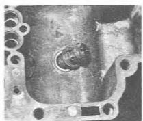
6.16 Removing the full power valve (DGAS type)
