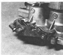
5.44a Removing the primary throttle shaft lever ...
