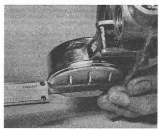
7.42 Checking the float closed position with vernier calipers
