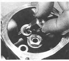
9.16B Removing the needle valve seat
