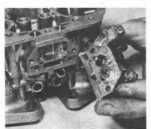
5.11 Removing the starter device
