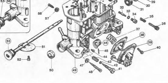
pull the main jets (11) and air corrector jets (9) from the emulsion tubes (10) (photo). Take care not to damage the jets when removing them and, if pliers are used, interpose a piece of paper or card to prevent the brass being scratched.
