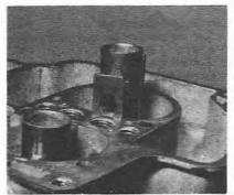
5.32a Removing an auxiliary venturi
