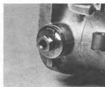
5.29 Throttle spindle end nut location and locktab
