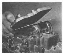
5.5 Lifting the carburettor cover
