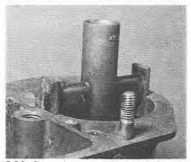
6.26a Removing an auxiliary venturi (triple choke type)
