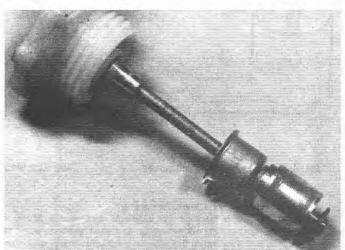
Fig. 4.27 Removing the damper rod
