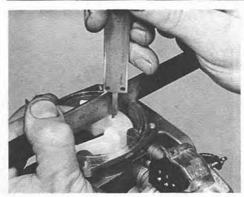
10.14 Checking the float level dimension
