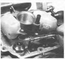
Fig. 4.18 Float removal on a typical Stromberg carburetor
