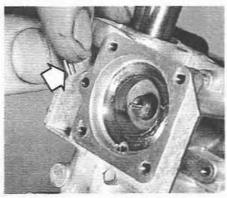
6.12D ... and locating dowel (arrowed)
