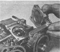
5.20 Withdrawing the accelerator pump cover from the carburettor
