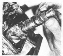
10.6/8 We assembled the jet complete before the float chamber cover. Follow the text
