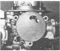
5.29a Location of the automatic choke disc gasket (DFAV type shown)
