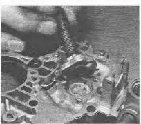
5.8 Removing the full power valve assembly
