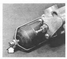
5.5 Cover retaining screw (arrowed) and locknut
