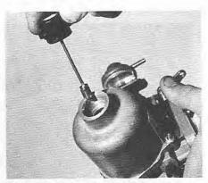
9.4A Removing the damper rod
