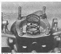
9.23a Fitting the accelerator pump return spring (triple choke type)
