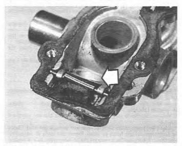
11.24 Air valve location (arrowed)
