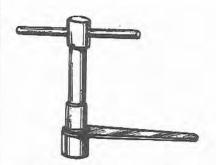
Fig. 11.18 Throttle spindle nut tightening tool (Sec 7)
