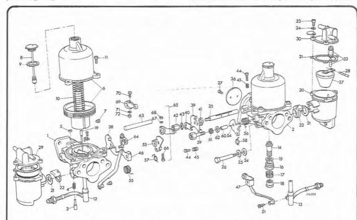
Fig. 7.5 Exploded view of twin HS4 carburettor installation (Sec 7)
