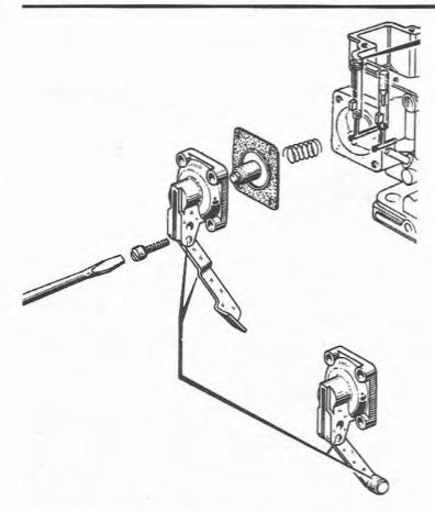
Fig. 7.18 Location of the accelerator pump inlet ball valve (Sec 6)
