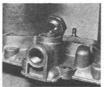
5.4 Removing the fuel filter (twin choke type)
