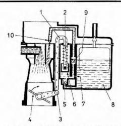
Fig. 1.7 The Weber piston type accelerator pump
