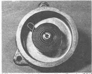
9.63 Automatic choke thermostat bi-metallic spring (DGAS type)
