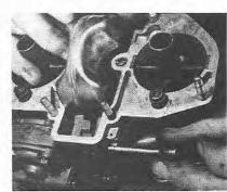
6.11 Removing the float fulcrum pin (triple choke type)
