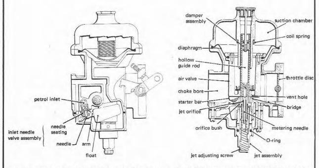
Fig. CD3 Cross-section of the inlet valve of the Series CD carburettor
