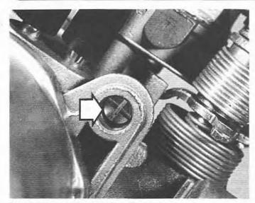
14.3 Throttle adjusting screw location (arrowed)
