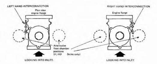
Fig. 1.13 Float chamber positions on the SU carburetors
