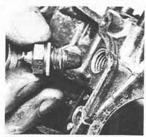
10.4 Use a new aluminium washer for the needle valve
