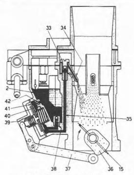
Fig. 12.4 Acceleration phase (Sec 3)
