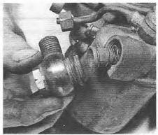
7.1 Removing the filter and spring assembly
