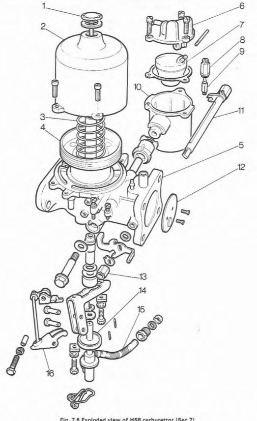
Fig. 7.6 Exploded view of HS8 carburettor (Sec 7)
