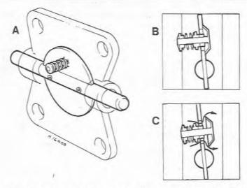
Fig. 7.1 Diagram of overrun valve fitted to throttle valve (Sec 1)
