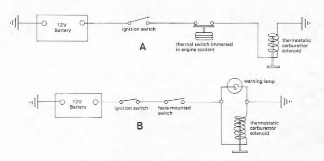
Fig. 9.5 Auxiliary enrichment device wiring diagrams (Sec 3)
