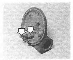
7.13 Needle and needle valve seating (arrowed)
