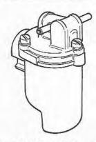
Fig. 4.19 SU type HS float chamber
