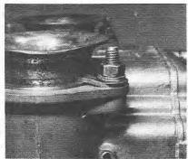
5.3 Air horn retaining nuts
