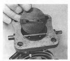
7.20B ... and lift out the throttle disc
