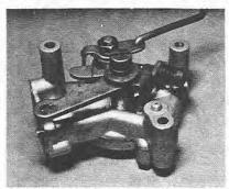
5.36 Automatic choke control levers (DFAV type shown)
