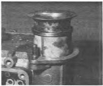
7.49 Fitting an air intake horn
