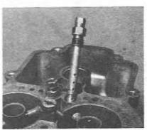
5.15a Removing an emulsion tube assembly
