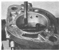
5.31 Removing the throttle valve retaining screws
