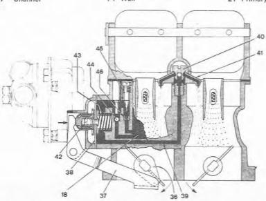
Fig. 9.7 Carburettor acceleration phase (Sec 3)
