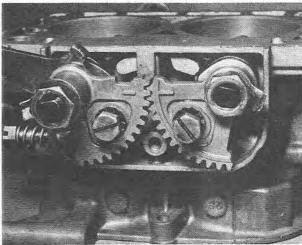
8.11 Fitting the sector adjustment screws (DFAV type)
