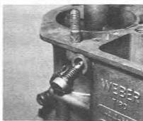
6.15a Removing an idling jet (triple choke type)
