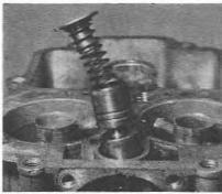
5.24a Removing the starting valve components
