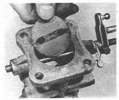
6.17C ... and withdraw the throttle disc
