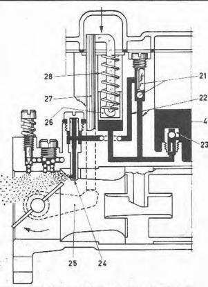
Fig. 11.10 Carburettor acceleration phase (Sec 3)
