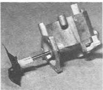
5.14a Withdrawing the electric choke operating rod
