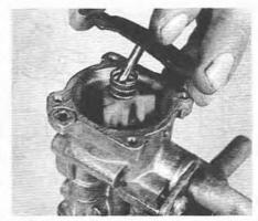
13.9A Remove the accelerator pump diaphragm ...
